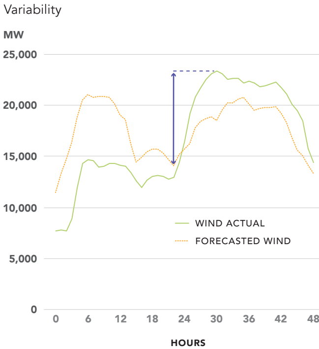
FIG 7 Example of the Variability of a Wind Plant and the Uncertainty of a Solar Plant 21
